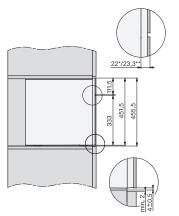
CVA7000, side view (\*footnote) (installation drawing) 22 mm - Glass, 23,3 mm - Cleansteel
