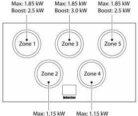
Max: 1.15 kW Max: 1.15 kW Boost: 2.0 kW Boost: 2.0 kW
